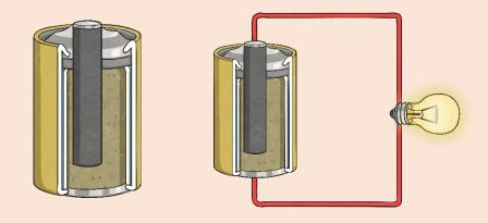
An electrolyte is a chemical that reacts with the electrodes to produce an electrical current.
