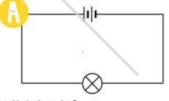
Is this circuit complete? Does the bulb work? Why is it not practical? How many cells are there in the battery?
